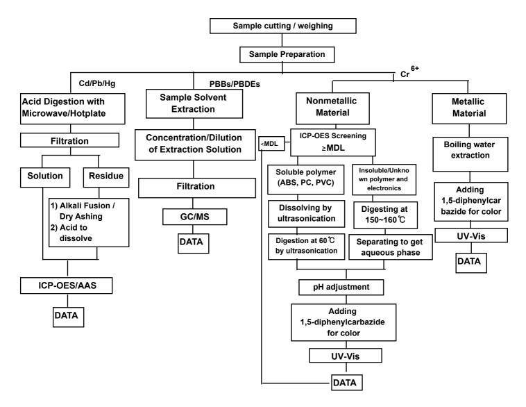
The samples were dissolved totally at the acid digestion step of the above flow chart for Cd,Pb,Hg Section Chief : Tonny Park
